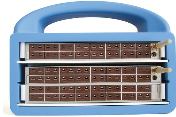
**48-thermocouple temperature measurement pack for real time temperature measurement at various points for thermal process control.**
