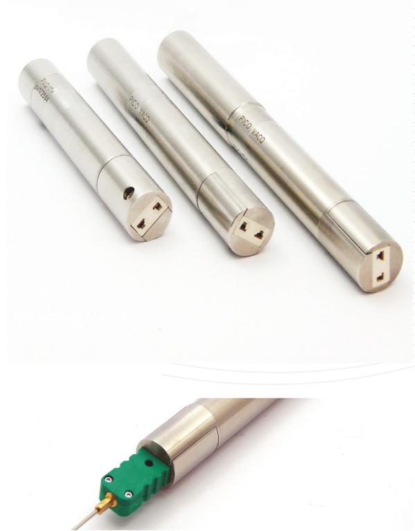
Temperature measurement in thermal processes up to +1820°C with an extra small thermocouple logger.
