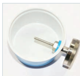
Examples of NanoVACQ Flat Needle positioning in containers
