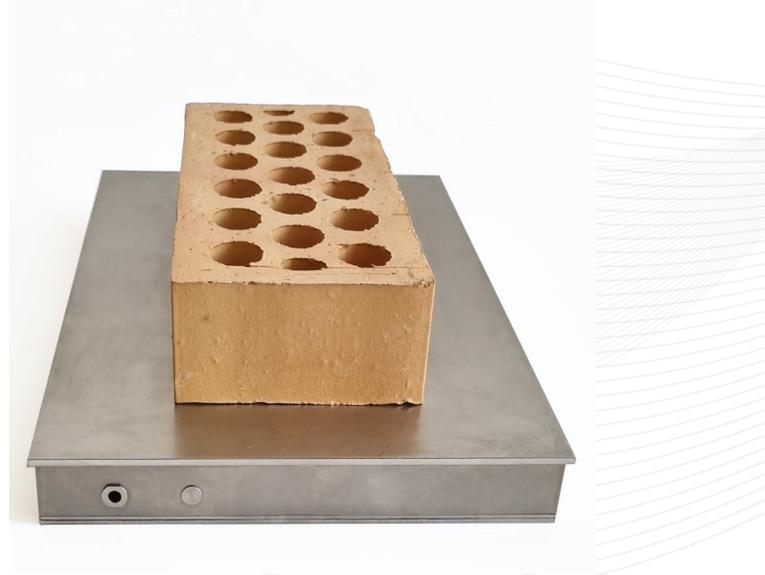
DryBal is a 3 cm high scale which logs mass variations in bricks, tiles or ceramics during drying processes.
