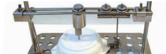
**Measurement of the deformation and dimensional variations of containers during thermal processes.**
