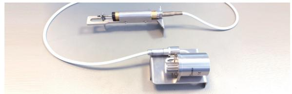
The CeriDry Split correlates the changes in relative humidity and air temperature with the shrinkage of bricks, tiles or ceramics during the drying process. It also enables the acute evaluation of drying within two parts of the same brick or tile.
